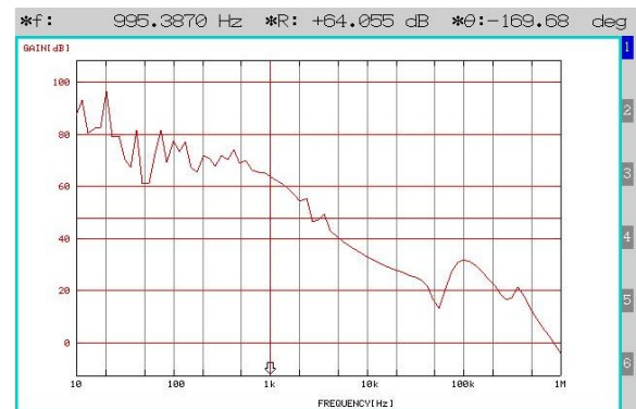
Fig 12. PSRR vs Frequency ( V_{IN}=4.8V , V_{OUT}=1.8V )
