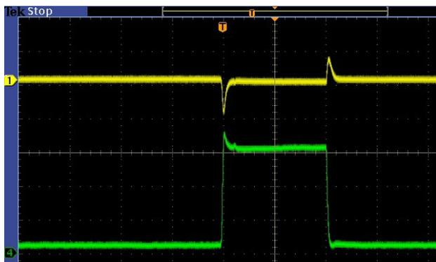
Fig 5. Vout Load Transient(1 to 150mA)
